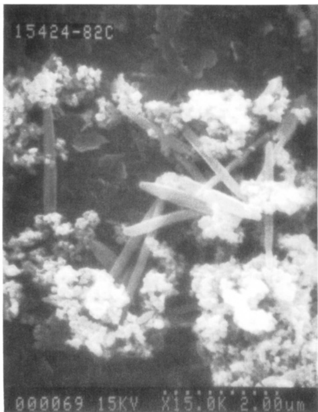
Figure 6. Scanning electron micrograph of pH 6 precipitated material following drying at 110 °C.
